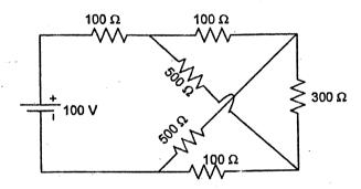
b) Obtain the voltages at each nodes by applying nodal voltage analysis.
