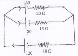
b) Find the current in the 10  $\Omega$  resistor in the circuit below using Superposition theorem. [6]
