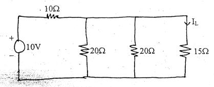
3. a) Use nodal method to find the current through  $10\Omega$  resistor for circuit shown below.
