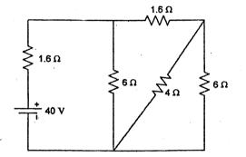
2. a) State and explain Kirchoff's laws. Determine the current supplied by the battery in the circuit shown in figure below.
