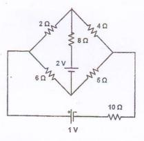
b) Use nodal analysis to find the current through  $6\Omega$  resistor for the network shown below.
