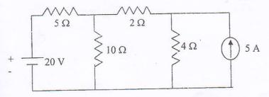
b) State the maximum power transfer theorem and find the value of R<sub>L</sub> to obtain the maximum in R<sub>L</sub> power and also find the value of this maximum power for the network shown below.
