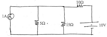
b) Determine the current I<sub>L</sub> through  $15\Omega$  resistor in the network by Norton's theorem.
