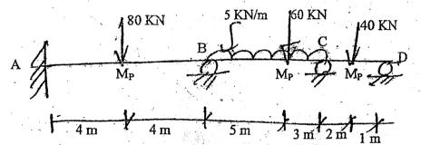
a) Using Castigliano's theorem, determine the moment at the fixed support A of the propped cantilever beam loaded as shown in figure below. [6]
