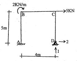
73. a) Generate stiffness matrix for the frame shown in figure below with respect to coordinates 1, 2 and 3 and use it to analyse the frame if the forces 5KNm and 4KN are acting at coordinates 1 and 3 respectively in addition to the external loads as shown in figure below. Take EI is constant for all members.
