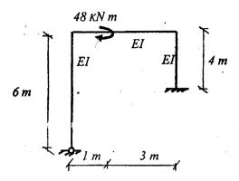
6. a) Determine Stiffness matrix for the frame shown in figure below.
