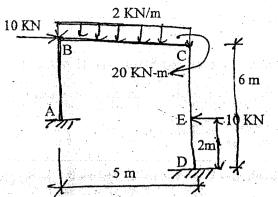
b) Analyse the frame shown in figure below by using moment distribution method. Draw bending moment diagram.
