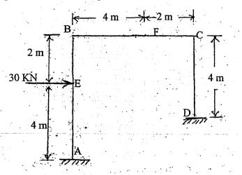
3. a) Analyse the frame shown in figure below by using stiffness matrix method and draw bending moment diagram. [10]
