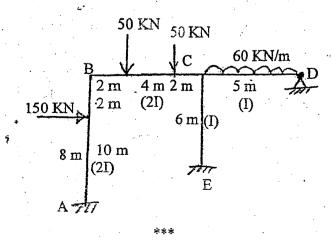
A continuous beam is shown in figure support 'B' sinks by 10mm down and 'C' rises by 20 mm up during loads. Analyse the given beam using slope deflection method and also draw bending moment diagram and show deflected shape. [15]
