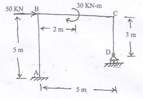
b) Analyse the continuous beam shown in figure below using slope deflection method. [10]
