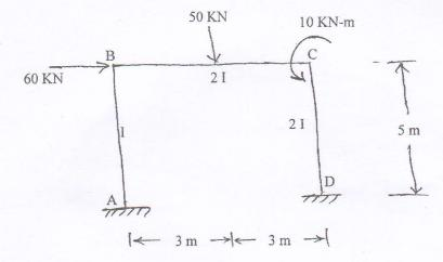
b) Determine the collapse load, W<sub>p</sub>, for the rectangular portal frame loaded as shown in figure below.
