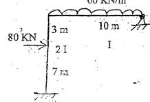
a) Analyse the frame shown in figure using stiffness matrix method. Consider only flexural deformations.
