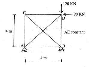
2. a) Draw shear force and bending moment diagrams for the frame given below. Use force [15] method.
