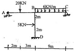
c) Use displacement method (Stiffness matrix) to find forces in members of the truss shown in figure below. Take axial stiffness for each member to be 400KNcm<sup>-1</sup>.
