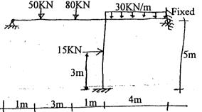
5. a) Define Muller-Breslau principle. Draw influence line diagram for reaction at C. Find ordinates at 2 m interval. [2+8]
