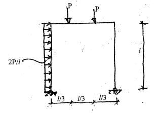
4. a) For the beam as shown, determine the slope at support B. Use Castiglano's second theorem. Take EI = constant.
