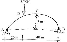
3. a) Generate stiffness matrix for the frame shown in figure below.
