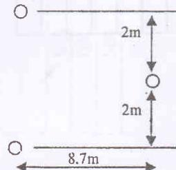
Assume: All towers are straight line towers. The air clearance is shown in figure. Minimum ground clearance is 6m. Neglect the effect of ground wire.
